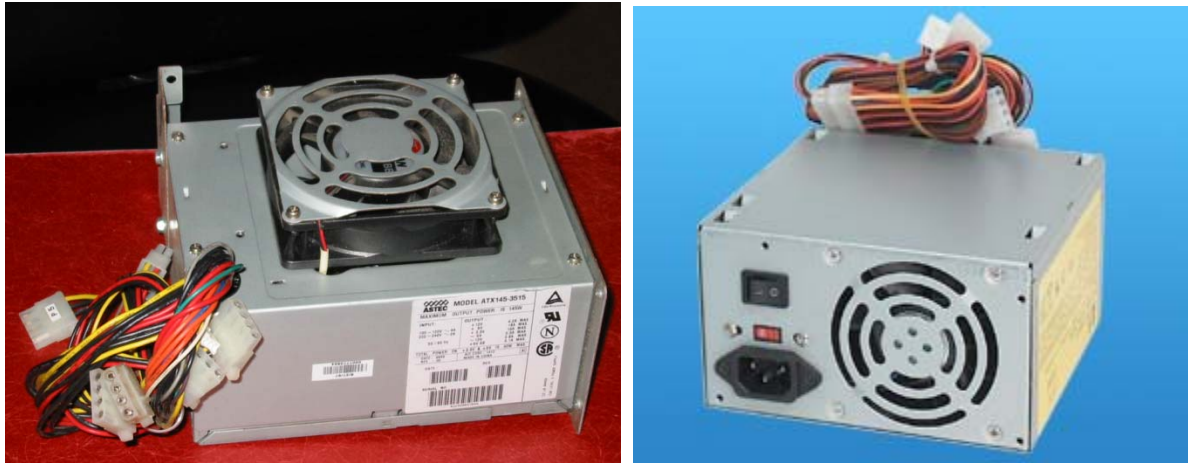
(a) Enclosed Frame Internal Power Supplies
