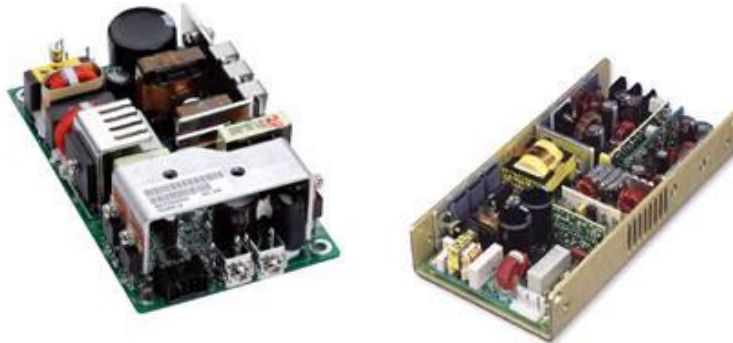
(b) Open-frame Internal Power Supplies
