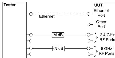
Figure 4: AP setup with removable antennas shown.
