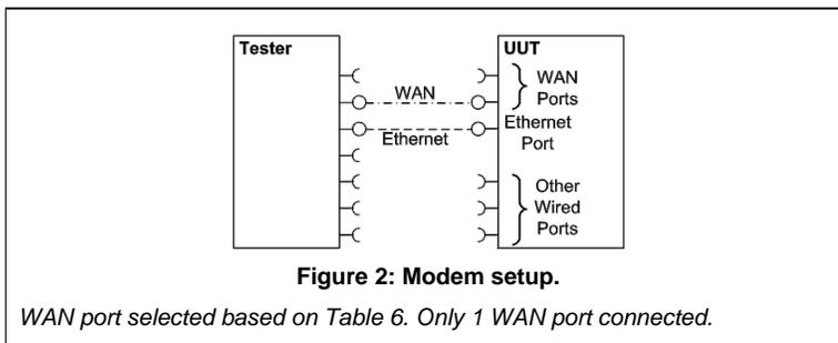
208 (a.) Connect the UUT WAN port to the test client using the priority and link rate specified in
