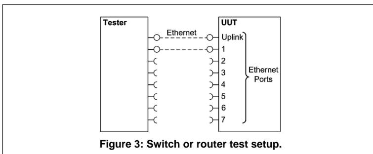
214 (a.) Connect two of the UUT's available ports to the test client and ensure that live links are
