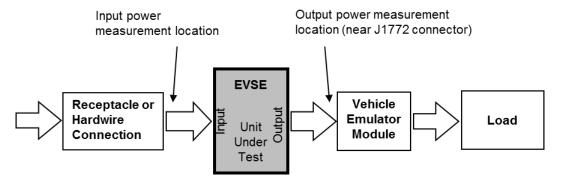
Figure 1a: Schematic of test setup connection
