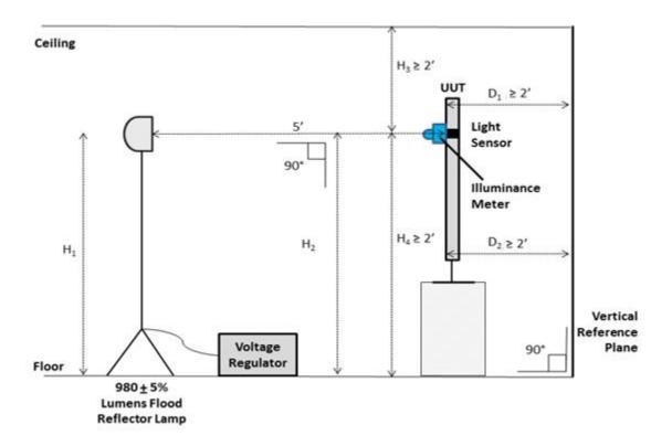
Figure 5: Test Setup - Side View
