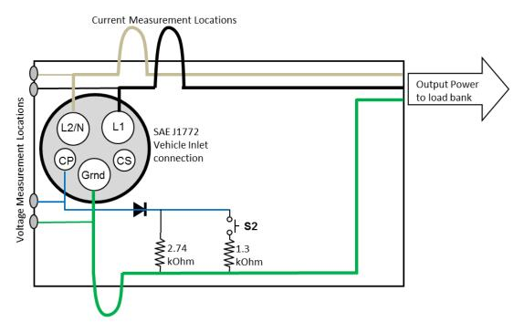
Figure 3: Schematic of Vehicle Emulator Module (VEM)<sup>2</sup>
