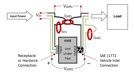
Figure 1b: Schematic of test setup connection
