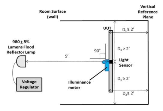
Figure 4: Test Setup - Top View
