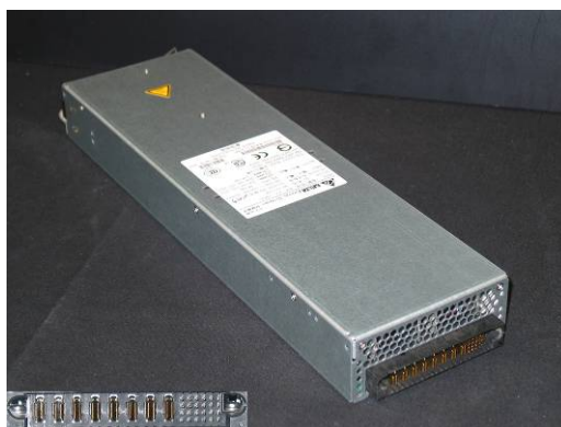
(c) 複数出力サーバ電源装置: 12VDC, 5VDC, 3.3VDC & -12VDC
