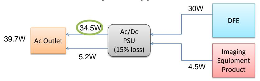
Imaging Equipment product and DFE share same power supply. By applying the same power supply loss to both, there is a 4.5W difference in the ac measurement.
